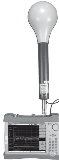
Cell Master MT8213E with 2000-1800-R Isotropic Antenna
