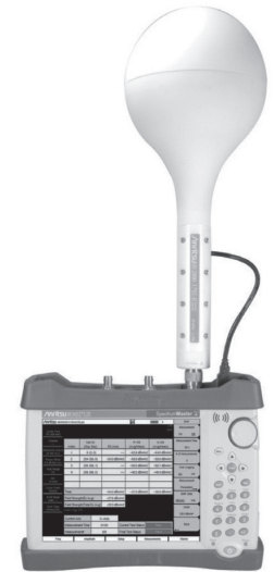
Spectrum Master MS2712E with 2000-1792-R Isotropic Antenna
