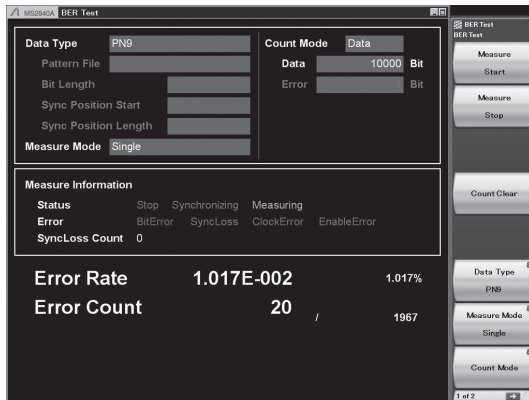
BER Measurement Function Main Screen
