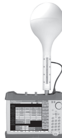
Spectrum Master MS2712E with 2000-1792-R Isotropic Antenna
