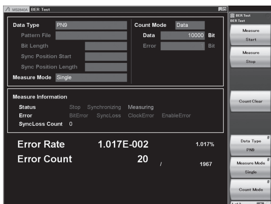
BER Measurement Function Main Screen
