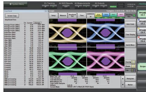
4ch NRZ Mask Margin Measurement
