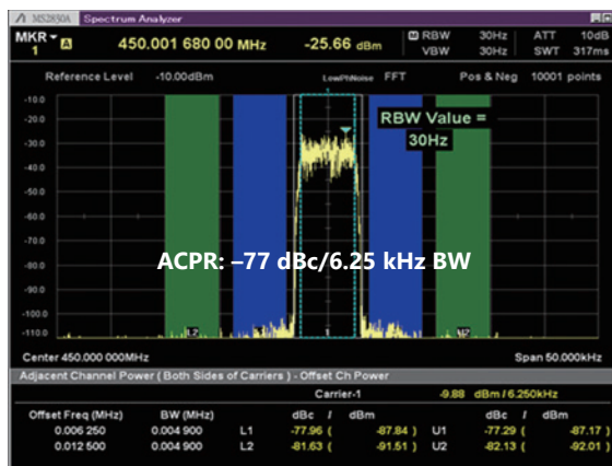
Example of ACPR Measurement (TIA-102/603)
