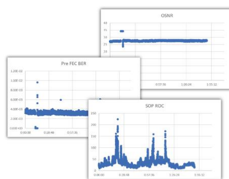
Example of continuous monitoring of media-side quality
