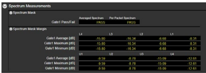
Figure 7-2: MT8862A Analysis Window – Spectrum Mask (Numeric Data)
