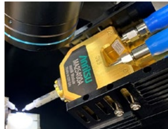
Dedicated probe tip (MA25400A + probe tip)
