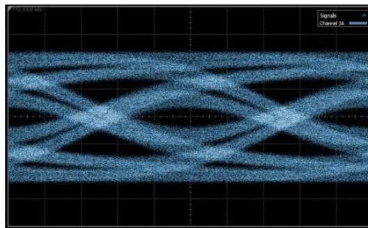
Fig. 4-3 Waveform A including ISI due to PCB frequency-dependent loss
