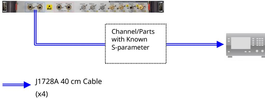
Fig. 4-2 Equipment Setup
