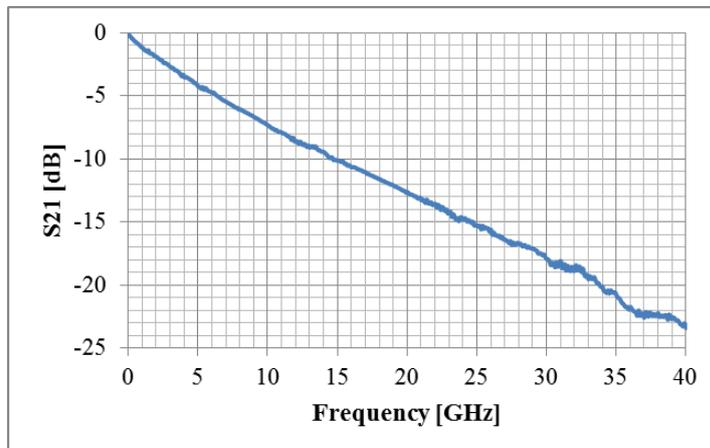
Fig. 4-1 6 dB at 8 GHz S21 Data
