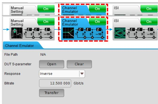
Fig. 3.1-1 Channel Emulator Setting Tab
