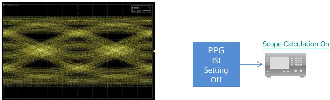
Fig. 2.3-4 Example of Adding Same 14 dB Loss to PPG (ISI Off) Waveform with Oscilloscope Simulation
