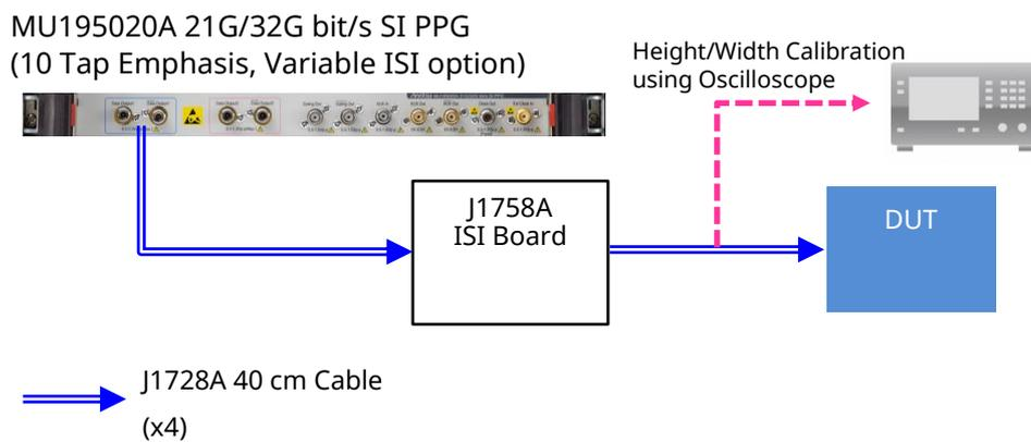
Fig. 2.2-1 ISI Addition Connection Cable
