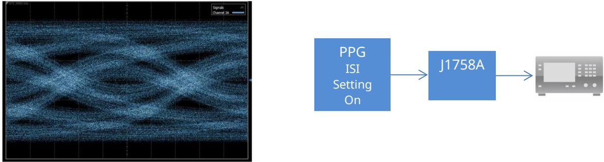
Fig. 2.3-3 Reference ISI Output Waveform
