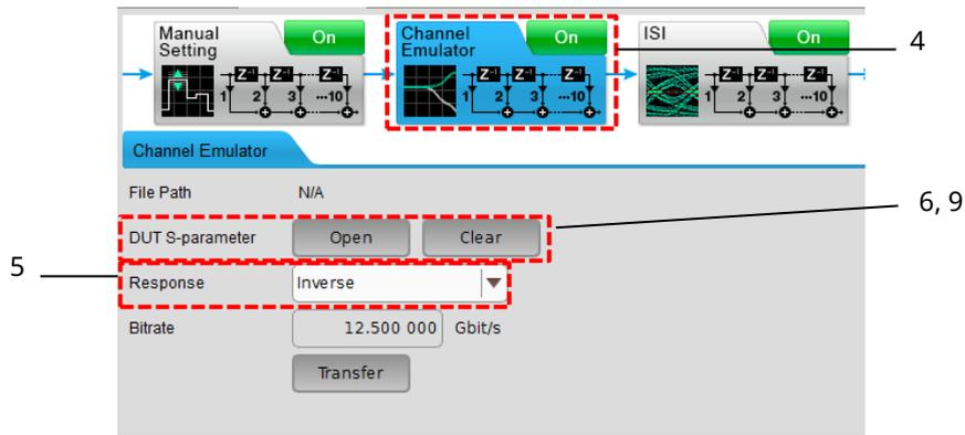
Fig. 3.3-1 Channel Emulator Setting Screen
