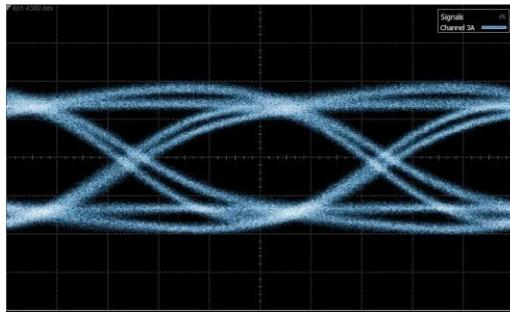
Fig. 4-5 Waveform B: EYE waveform after correction for frequency-dependent loss using inverse of loaded S-parameter
