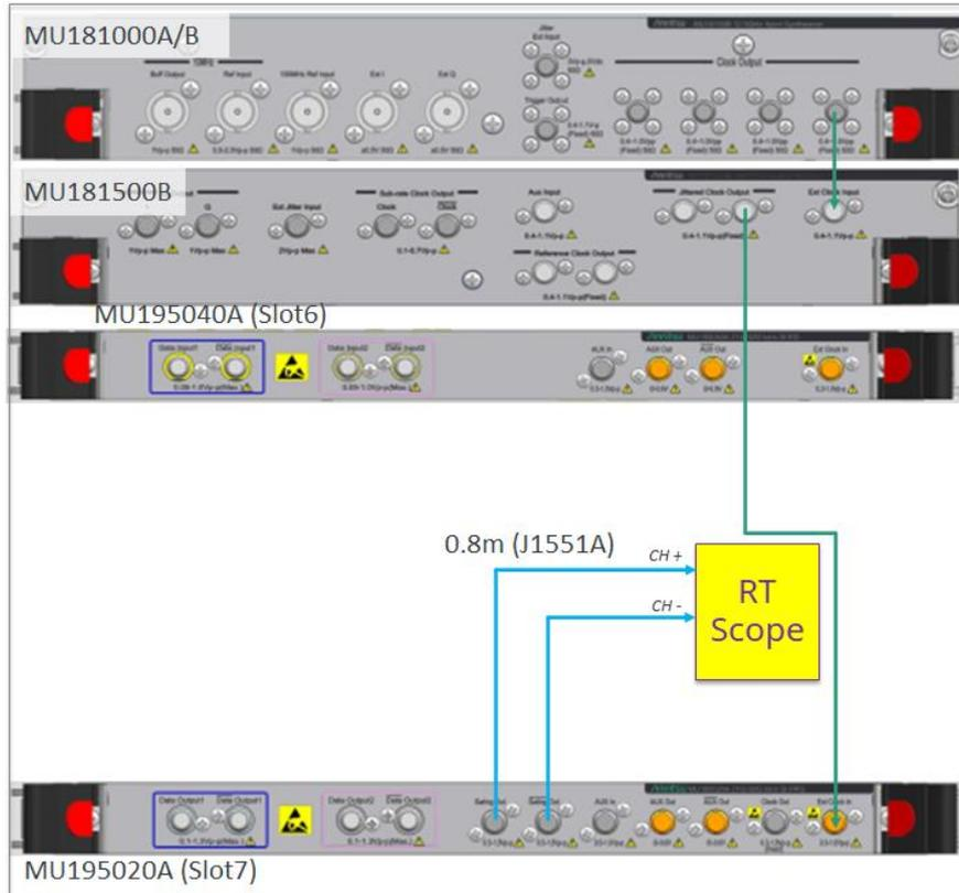
Figure 3.1.1-1 1000 mVpp/1200 mVpp LFPS signal calibration connection
