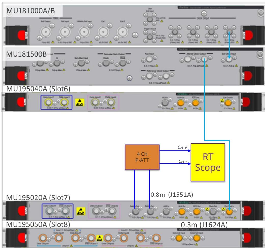
Figure 3.2.1-1 90/100/200/300/800 mVpp LFPS signal calibration connection
