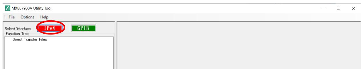
Click **IPv4** to display the Network interface selection screen showing the IP address configured in section 2.4.
