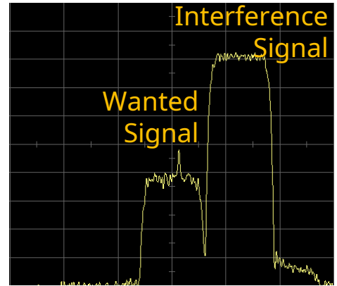
Output Signal Image (Example of Confirmation using Spectrum Analyzer)
