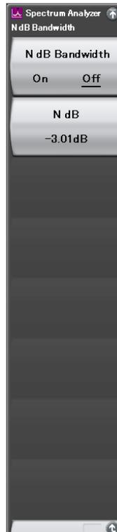
Sets N dB Bandwidth measurement function On/Off
