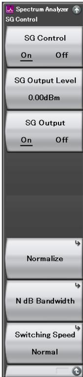
Sets Internal Signal Generator Control Function On/Off
