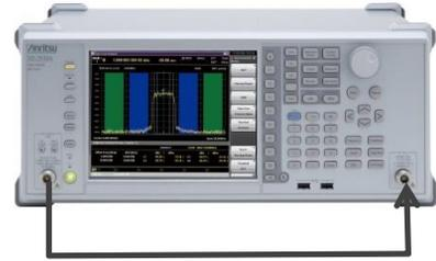
First, output an unmodulated signal from the signal generator and adjust the offset for cable loss, etc.
