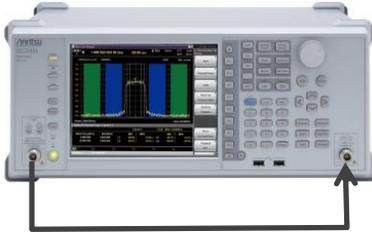
(1) First, output the following modulation signal from the vector signal generator option installed in the Signal Analyzer MS2830A and confirm the level and modulation accuracy (EVM) at the MS2830A.
