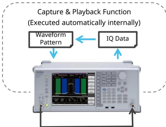
(2) Second, confirm the level and modulation accuracy (EVM) at the MS2830A for the modulation signal played back using the Capture & Playback function.
