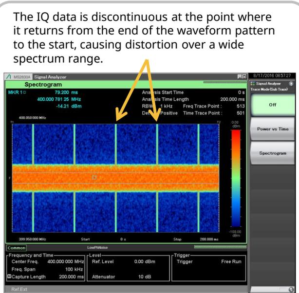
Example of Spectrogram Measurement Screen
