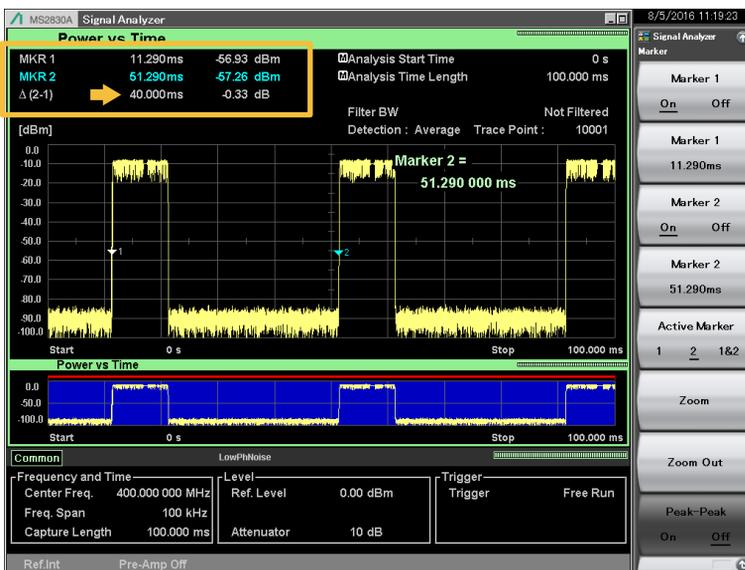
This sample signal has a period of 40 ms per burst that can be also checked with a signal analyzer.
