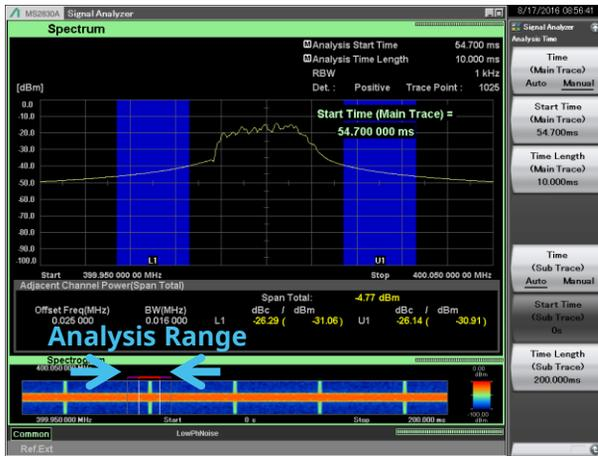
Example of Adjacent Channel Leakage Power Measurement Screen
