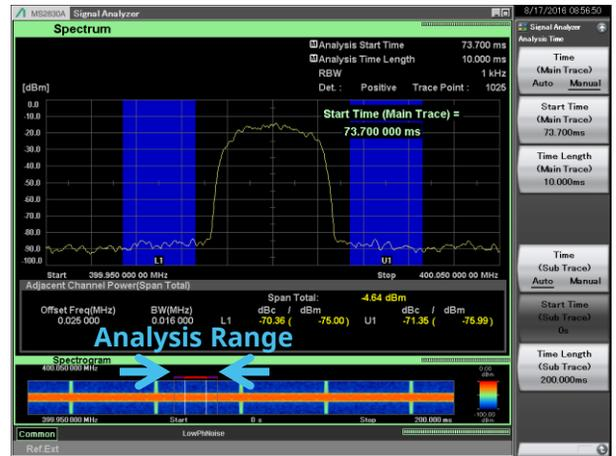
Example of Adjacent Channel Leakage Power Measurement Screen
