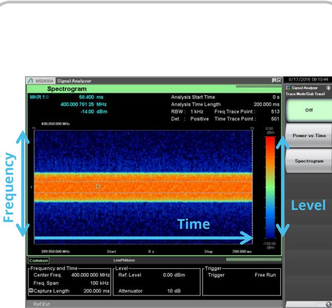
Example of Spectrogram Measurement Screen
