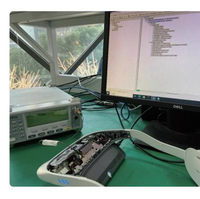
Like the WLAN testing product, the MT8852B also supports comprehensive versions of the Bluetooth protocols. "From the earliest Bluetooth basic data rate, through enhanced data rate testing specifications, the Bluetooth Low Energy (BLE) test specifications, to the latest RF testing specifications such as Bluetooth 4.2, 5.0, 5.1, 5.2, and 5.3. It is easy to operate, as everything is based on the testing specifications."
