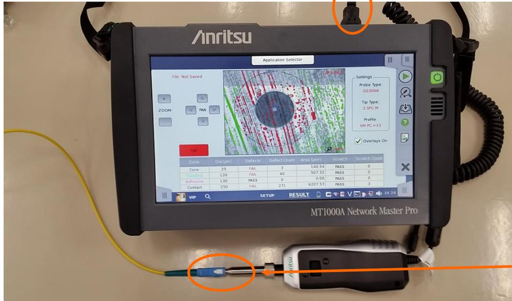
1. The VIP USB terminal is connected to the MT1000A/MT1040A series instrument's USB port.
