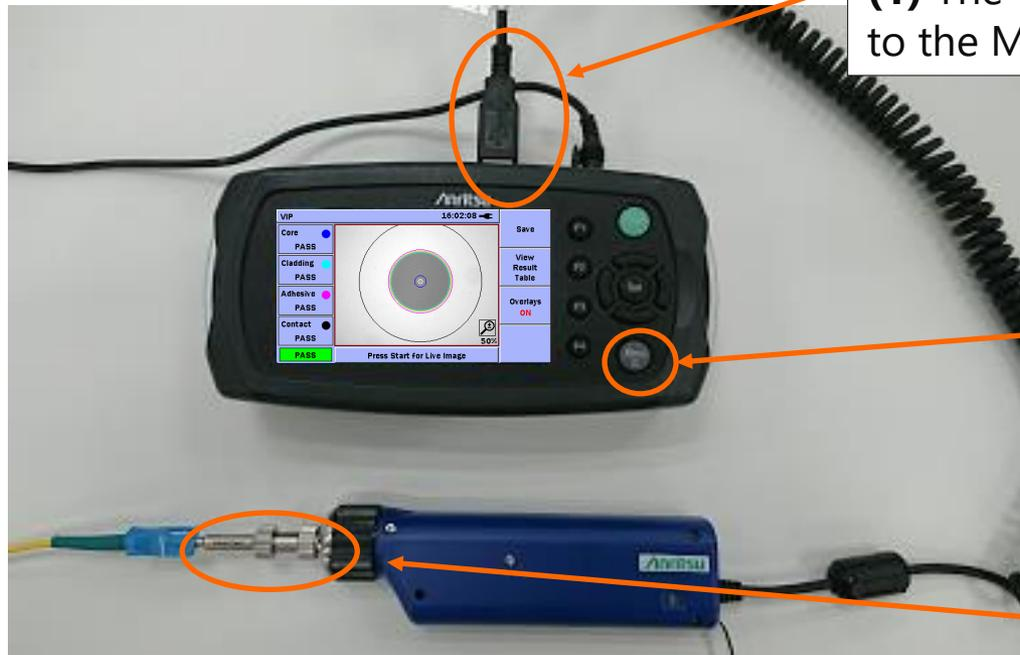
**(1)** The VIP USB terminal is connected to the MT9090A's USB port.
