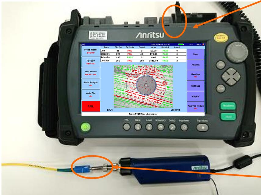
\*Before starting, select the appropriate tip for the connector adapter and ferrule type to be connected to.
