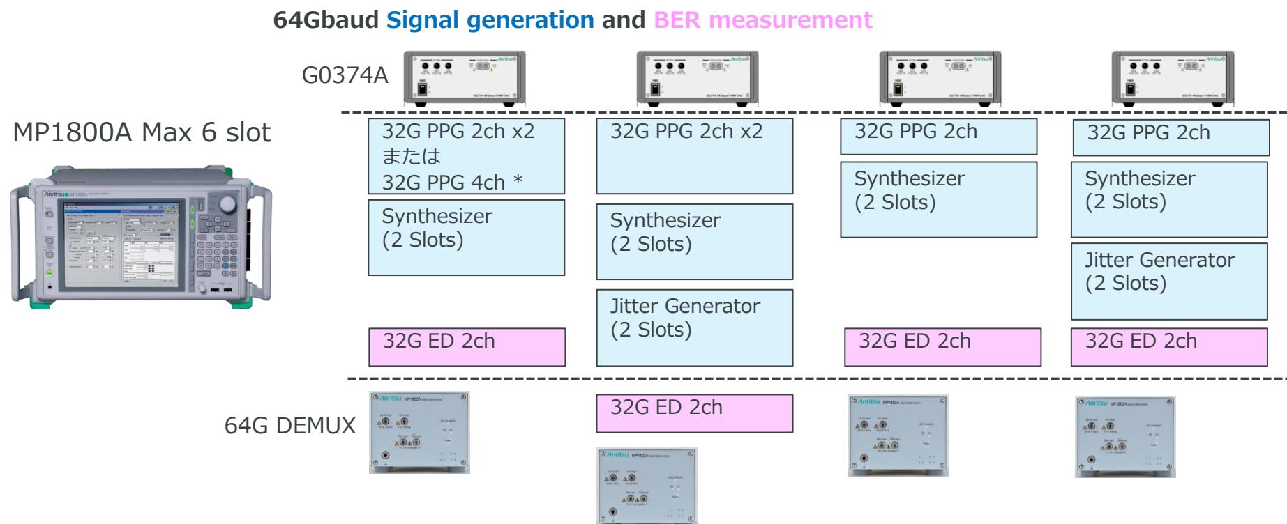
\*For Jitter addition, use the 32G PPG 2ch x 2 configuration as shown in slide 13.
