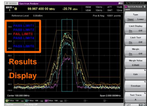
PASS/FAIL evaluation is performed by changing the input signal level. The evaluation results for the five line types can be displayed simultaneously on one screen.
