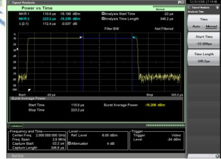
The Power vs. Time trace displays a graph with amplitude on the y-axis and time on the x-axis to confirm changes in power with time of measured signals.
