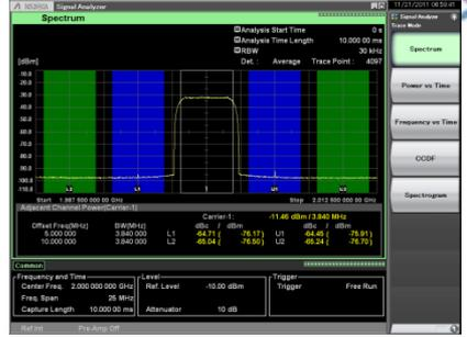
Displays waveform of wideband SPAN up to 125 MHz without interruption
