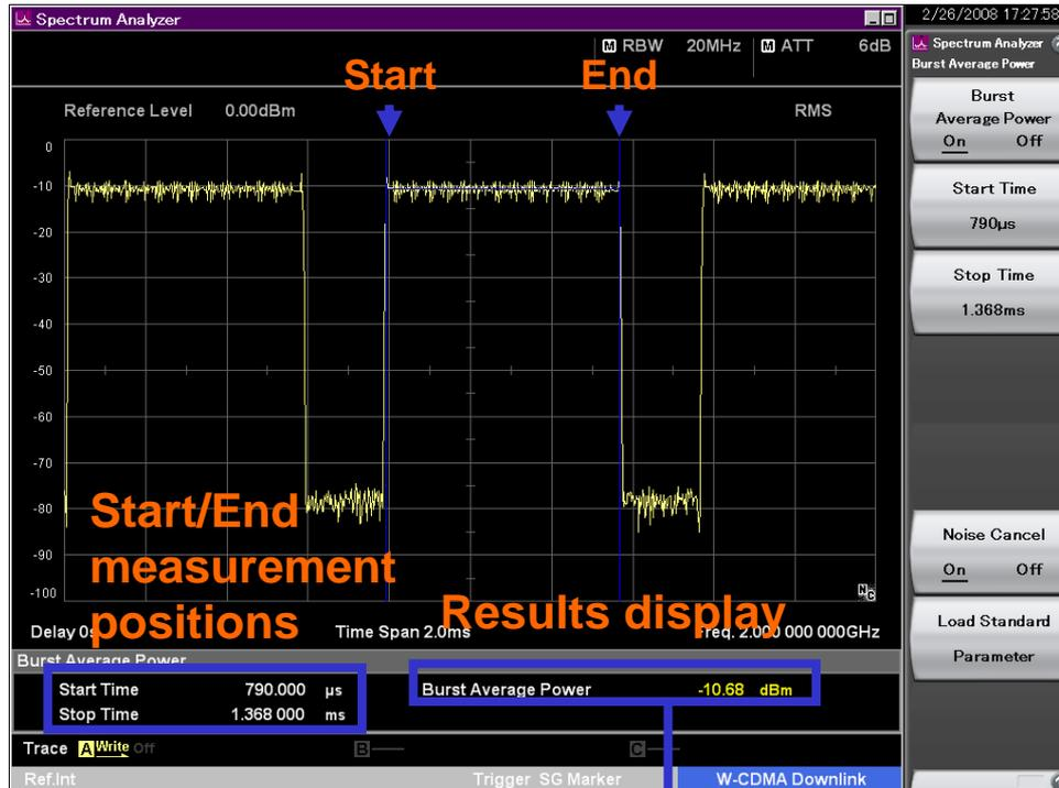
Burst Average Power Measurement function ON/OFF
