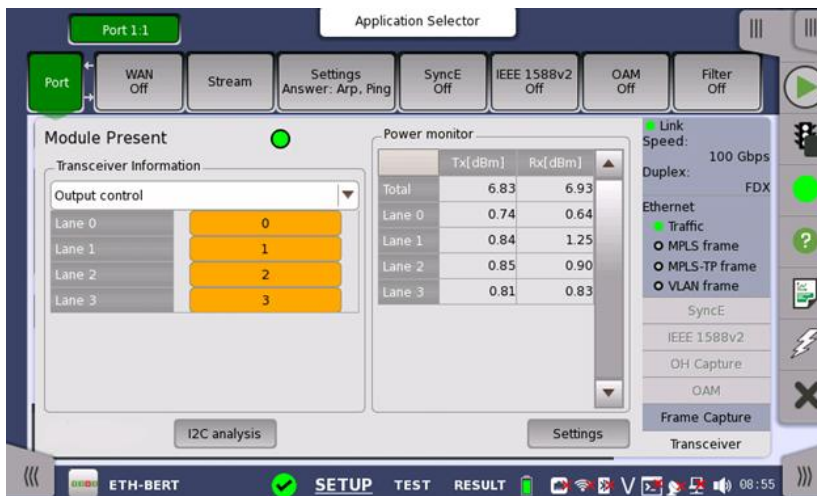
Example of Power meter and Power On/Off
