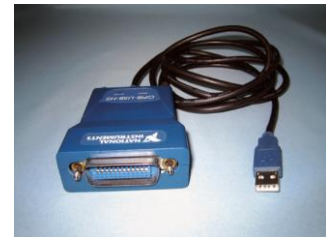
J1667A GPIB-USB Converter available for automated environments based on GPIB.
