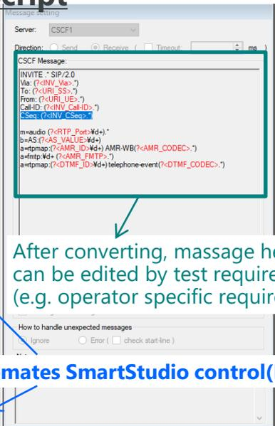
After converting, message header can be edited by test requirements (e.g. operator specific requirements)
