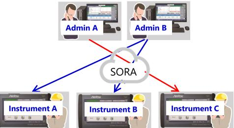
Administrator A remotely controls Instrument C while Administrator B remotely controls Instruments A and B. In this case, an additional option is required to remotely control the three instruments simultaneously.
