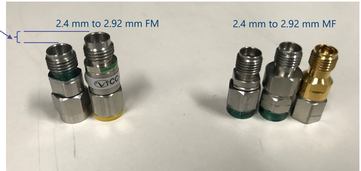
Adapters used in the lab for introducing skew
