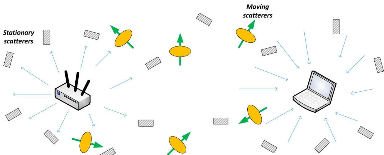
Figure 4: Scattering Environment for Wireless LAN
