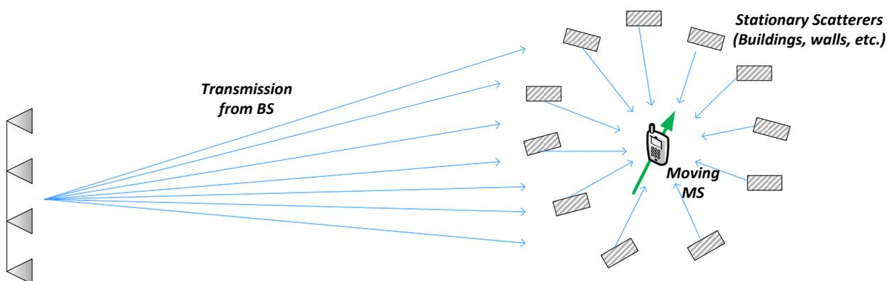
Figure 3: Scattering Environment for a mobile device
