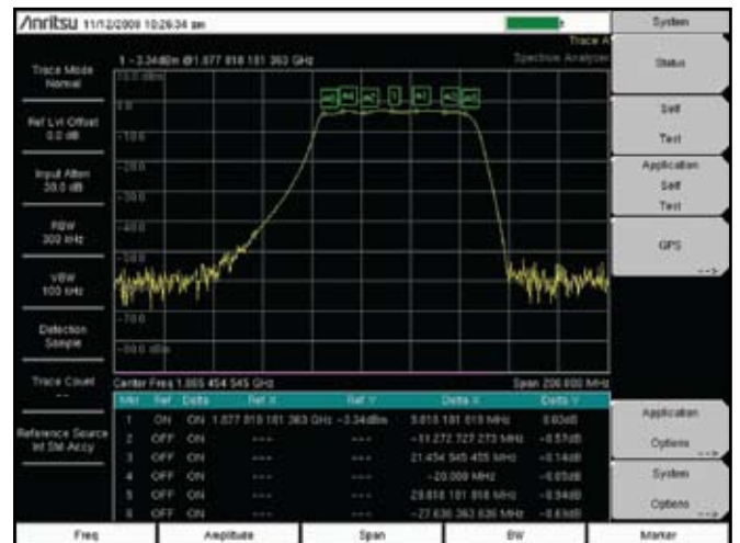
Figure 4. Filter passband after adjustment fixed and delta marker
