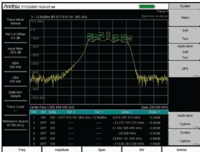
Figure 3. Measuring filter passband using fixed and delta markers.
