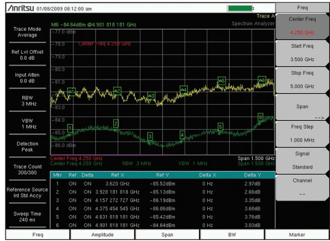
Figure 2. Noise figure measurement of a preamplifier with approximately 3.7 dB NF
