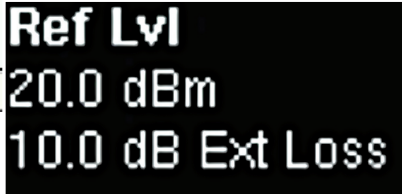
Figure 2. Annotation for Reference Level Offset, in this case 10 dB of External Loss which adds 10 dB to all measured power levels.
