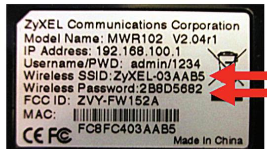
Figure 3. The Pocket Router configuration information.
