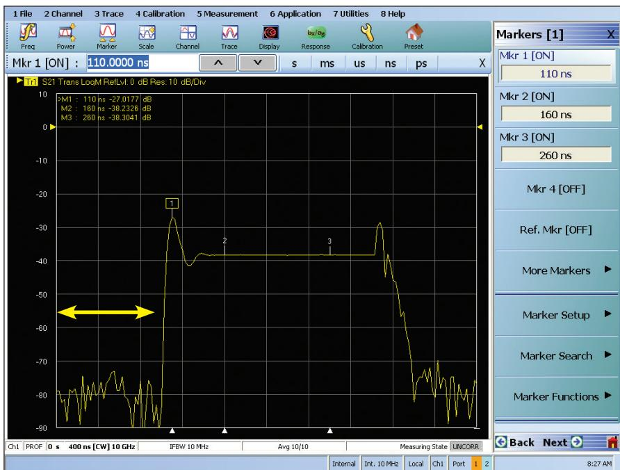
The pulse appears to be relatively flat beginning at ~160 ns for a duration of at least 100 ns (for convenient round numbers).
