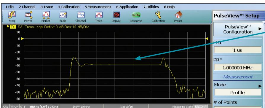
Example DUT measurement at 10 GHz displaying the effect of incident and reflected signals combining.
