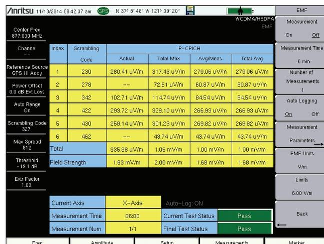
Figure 7. EMF result display for LTE measurements (similar to TD-LTE)
