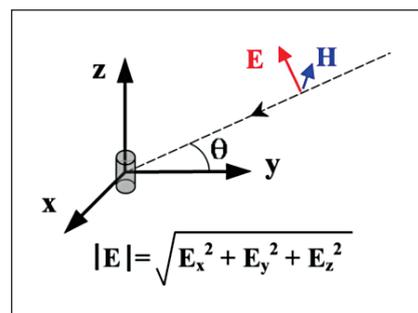
Figure 3. Antenna Configuration. Total measurement given by formula shown
