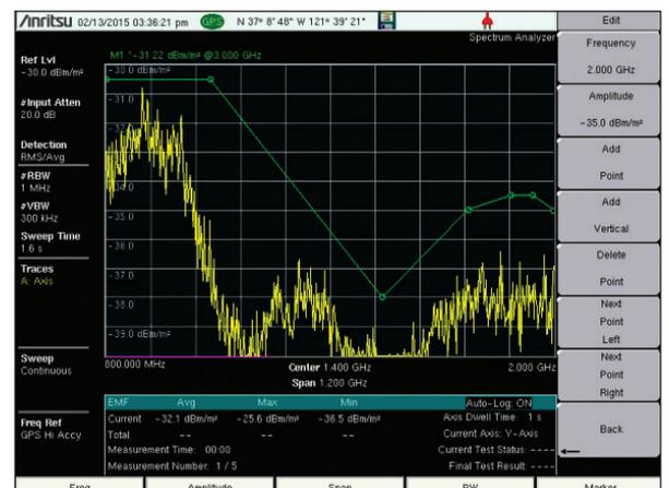
Figure 2. Wideband EMF measurement with limit line
