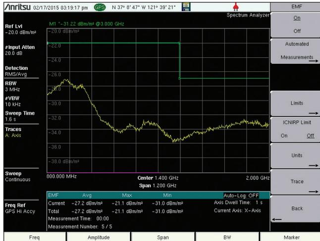
Figure 5. EMF result display in spectrum analyzer mode (broadband field strength measurements)
