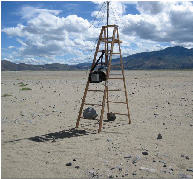
Figure 4: S412E with a WiFi router and omni directional antenna
