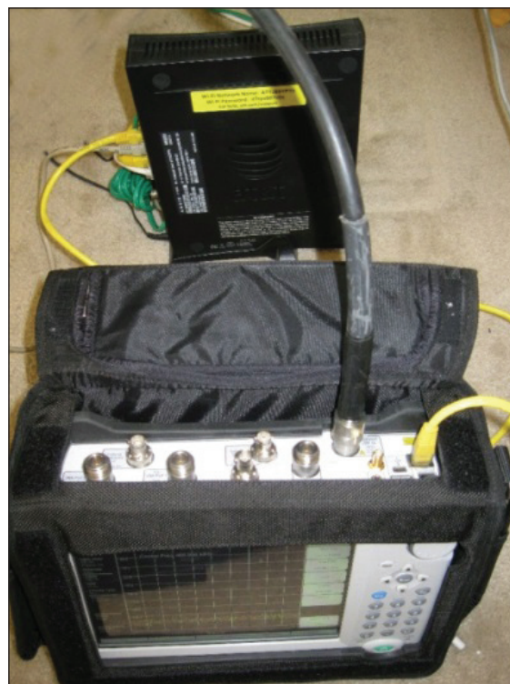
Figure 2: Showing the S412E connected to the internet through a router and an omnidirectional test antenna.
