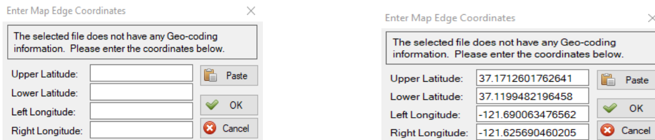
Figure 5. Window Where GPS Coordinates are Copied. The Picture on the Right Shows the Panel Populated with Coordinates.
