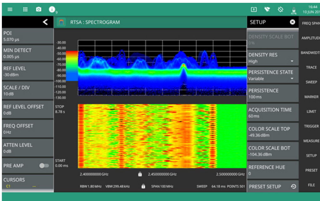
Figure 4. With the spectrogram display, the three Wi-Fi access points and 3 BLE advertising channels are clearly visible.
