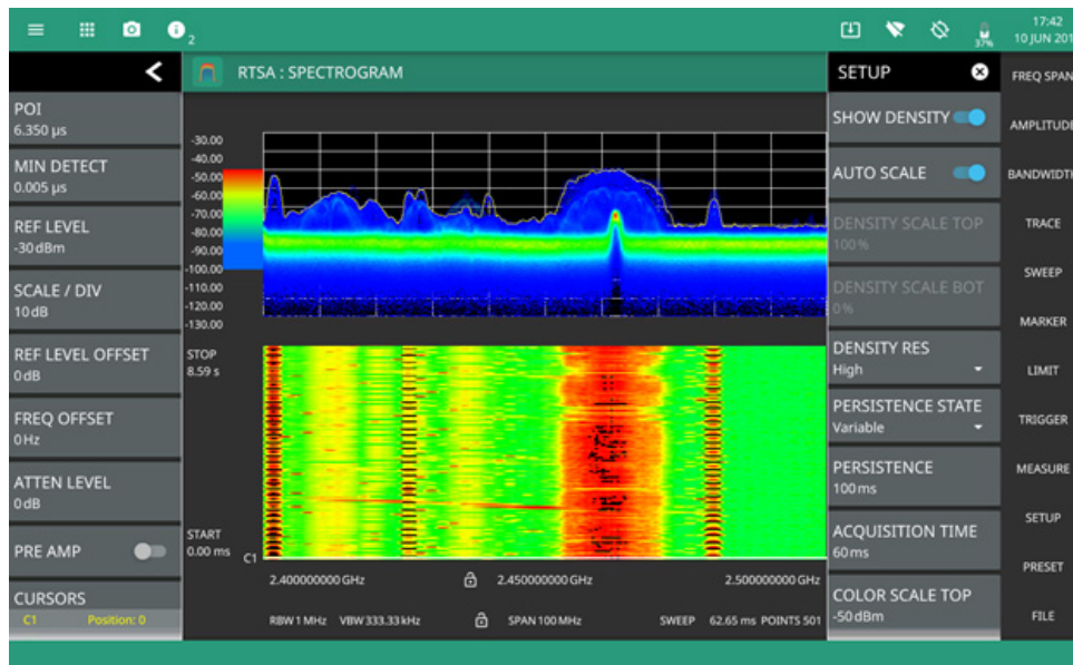
Figure 5. When transmitting data, the highest frequency Wi-Fi access point can be seen to be transmitting at an OFDM spectrum as opposed to the DSSS modulation used for beaconing.
