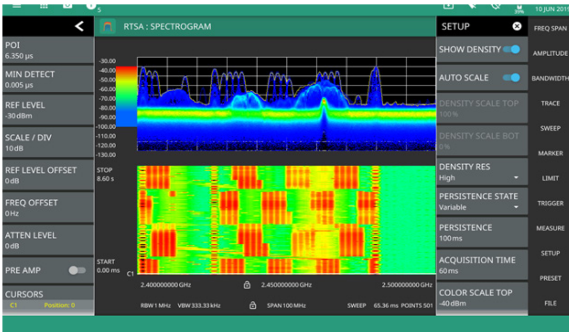
Figure 6. The Bluetooth inquiry scanning raster is clearly visible as the device searches for other Bluetooth devices in the area.
