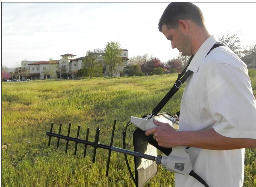
Figure 10. Final Step in Geo-Locating Interference Source
