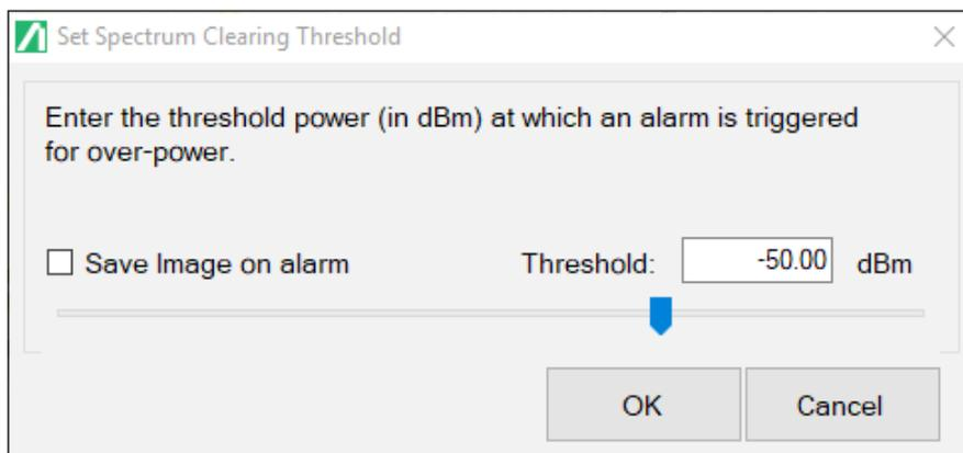
Figure 5. Spectrum Clearing Threshold Setting
