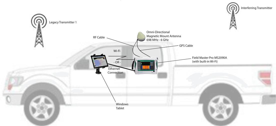
Figure 3: Spectrum Clearance and Interference Hunting Components
