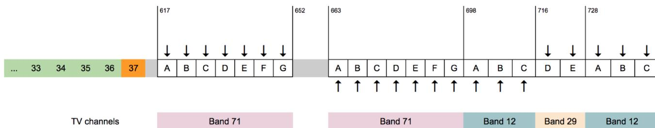
Figure 1. Spectrum for 600 MHz Deployments <sup>1</sup>
