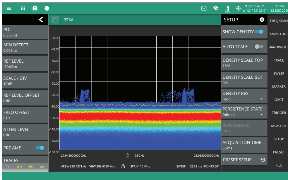
The Field Master Pro MS2090A RTSA Has an Infinite Persistence Setting to Capture any Signal Movement over a Long Period of Time During Spectrum Monitoring
