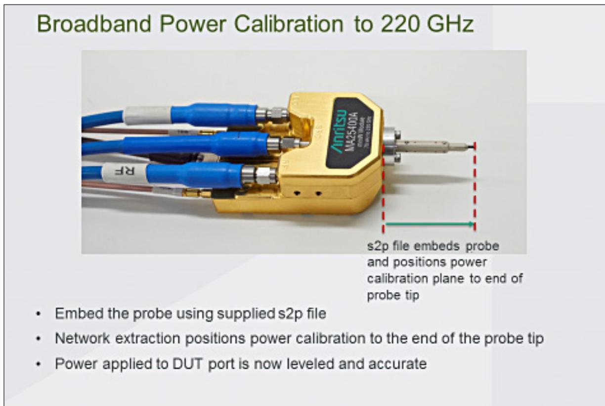
Figure 1. Embedding the probe for power calibration transfer
