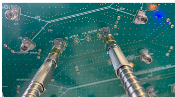
Figure 1: Picture of the transmission line with vias showing the cable connections. A V coaxial calibration was performed at the end of the cables
