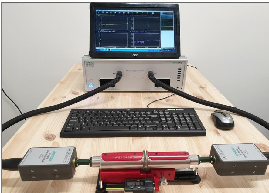
Figure 17: Example of a corrugated waveguide measurement
