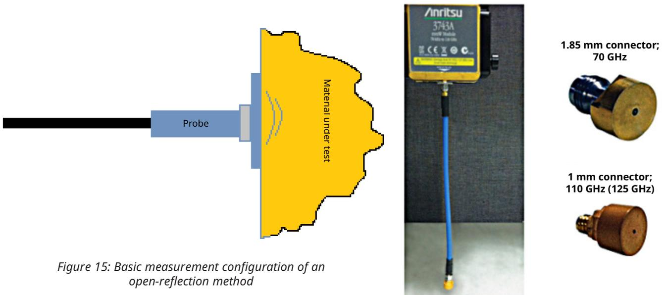
Figure 15: Basic measurement configuration of an open-reflection method
