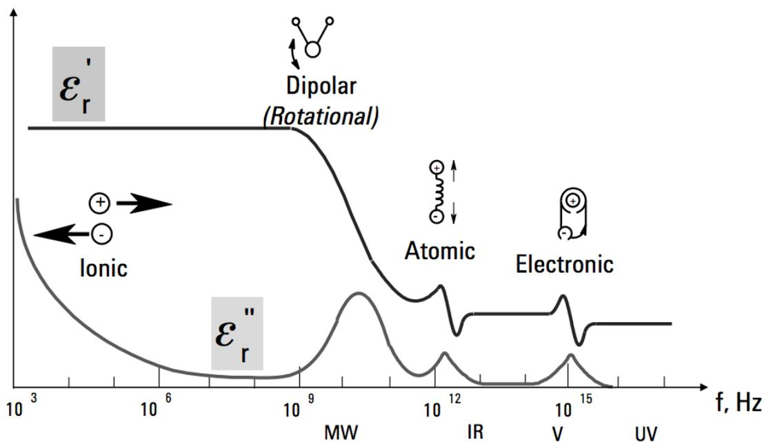
Figure 8: Various polarization phenomenon at different frequency ranges
