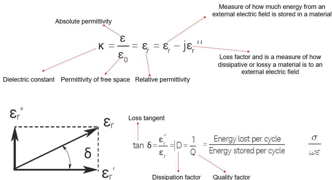
Figure 5: Material measurement - terms and parameters
