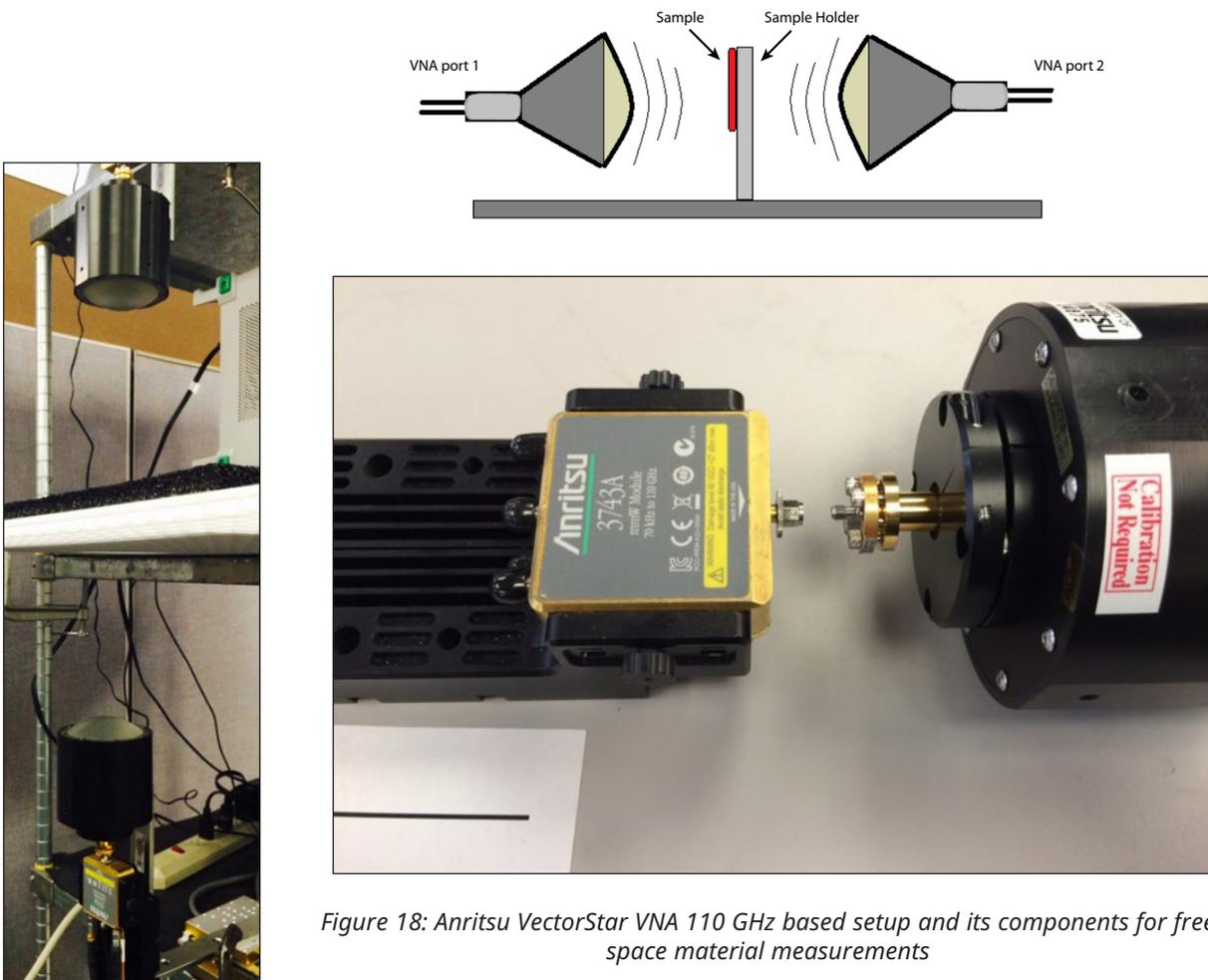
Figure 18: Anritsu VectorStar VNA 110 GHz based setup and its components for free space material measurements
