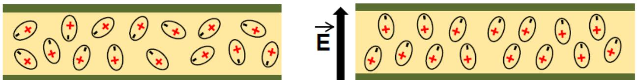
Figure 7: Polarization effect
