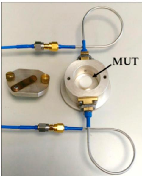
Figure 10: TE<sub>016</sub> mode cavity resonator
