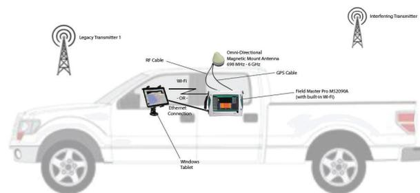
Figure 25. MIH Guides Driver to Signal Location
