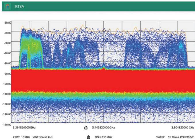
Figure 17. Cellular 5G Signal Centered at 3.45 GHz
