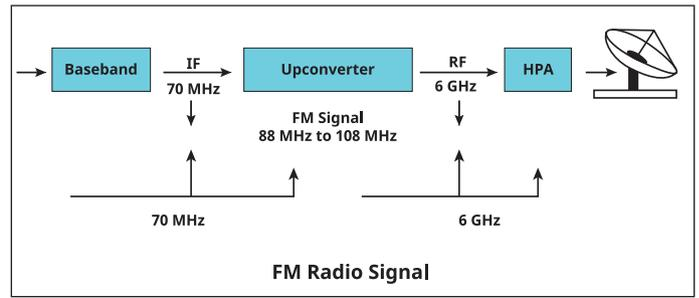
Figure 12. FM Signal Upconverter to Satellite Band
