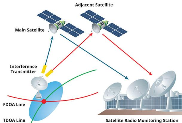
Figure 24. Satellites Using TDOA for Signal Geolocation. Inaccuracies of 10-20 km Often Result, Requiring Use of Mobile Interferencehunter to Pinpoint Interference Position
