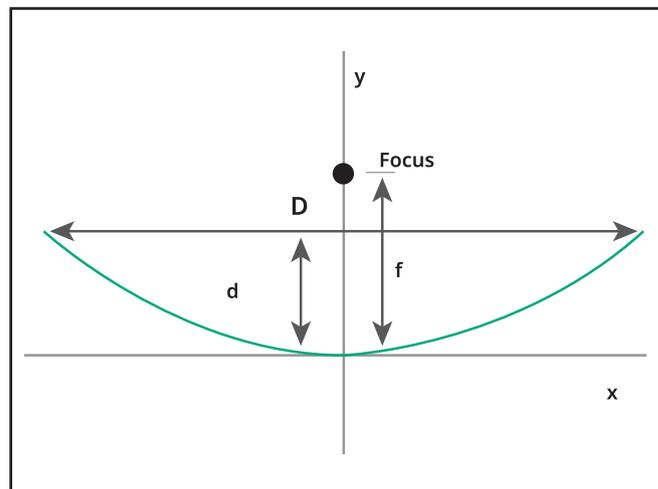
Figure 3. Distance Parameters for Antenna/Receiver System
