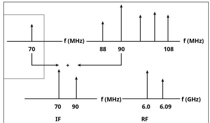
Figure 13. Intermodulation Signals (Interference) Shown
