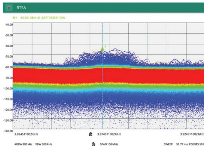
Figure 18. 5G Interference in Satellite Band
