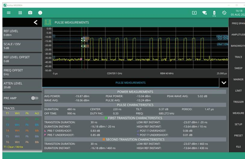
Figure 11. Field Master Pro MS2090A Pulse Analyzer Display
