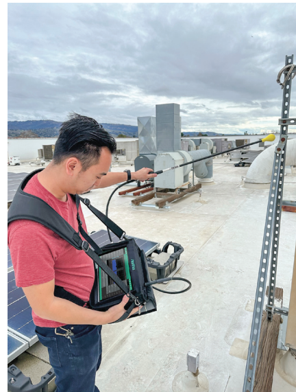
Figure 4. Technician Performing PIM Hunting Exercise with Anritsu Field Master Spectrum Analyzer and PIM Hunter Probe
