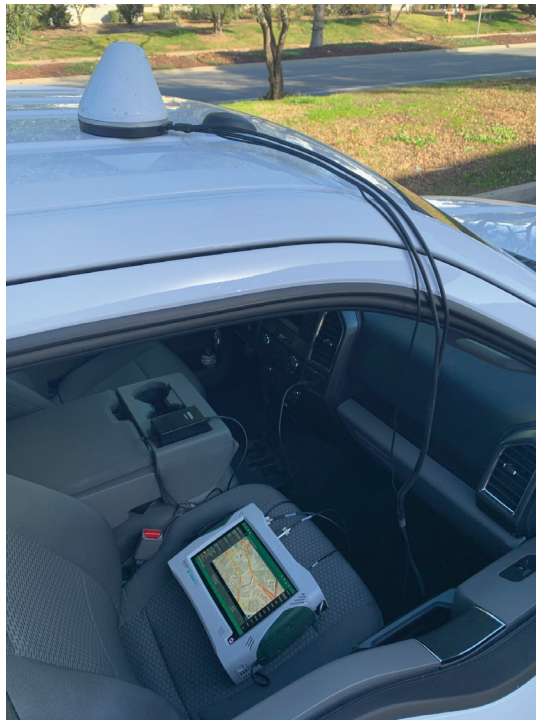
Field Master Pro MS2090A in a Vehicle with a Magnetic Mount Omnidirectional Antenna Connected to DC Power Supply
