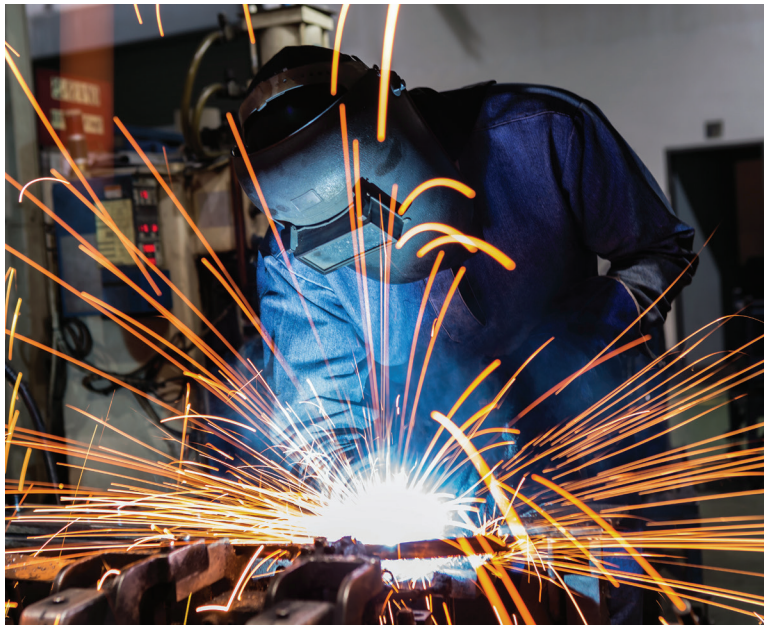
Figure 6. Arc Welders and other Heavy Industrial Processors can Create High Levels of RF Interference
