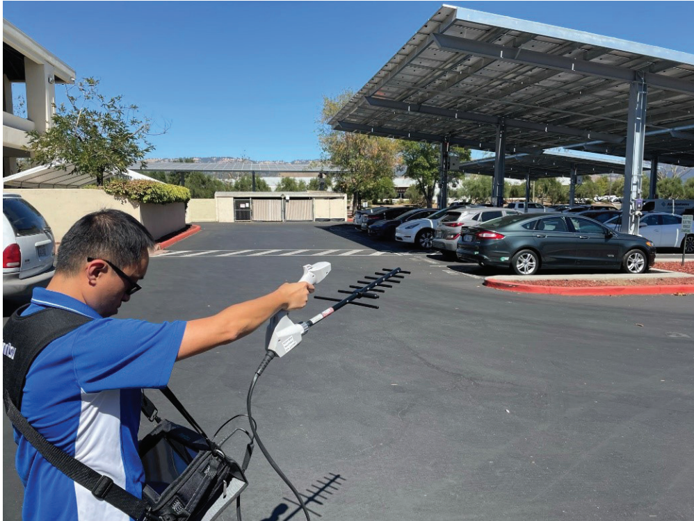
Figure 17. Using InterferenceHunter MA2700A to Direction Find an Interfering Source
