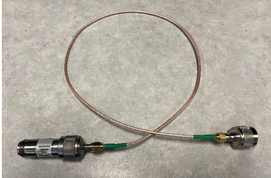
Figure 1. SMA Cable with Adaptors on Both Ends
