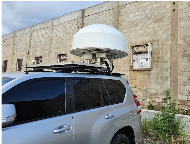
Figure 5. The SMA also has Two Vehicle-Mounted Monitoring Stations that Use Angle of Arrival (AOA) Technology to Pinpoint Interference Sources More Precisely
