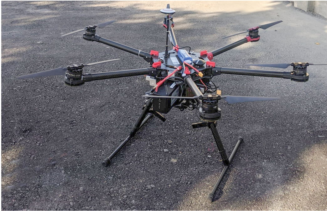
Figure 4. Drone Mounted with Anritsu MS2760A Ultra-Portable Spectrum Analyzer
