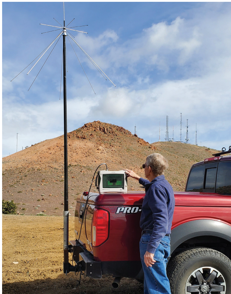
Figure 1. The Author Tom Brinkoetter from RadioSiteTest is Using the MS2090A with a 50 MHz to 1.2 GHz Discone Antenna to Survey a Busy Radio Site
