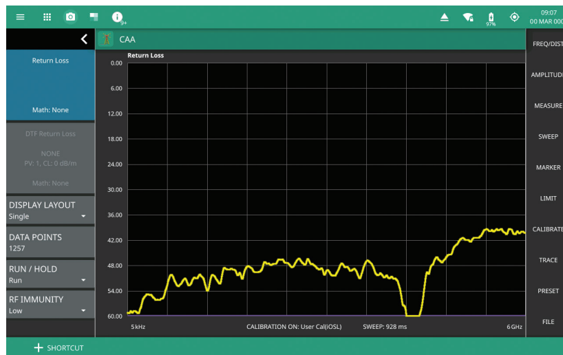
Figure 3. Measurement of the Precision Load following an InstaCal Calibration
