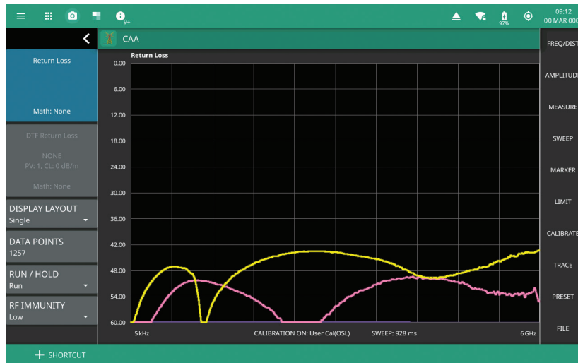
Figure 5. Comparison of Return Loss Measurement when Connecting a Precision Load Finger Tight (yellow trace) and Using a Torque Wrench (pink trace)
