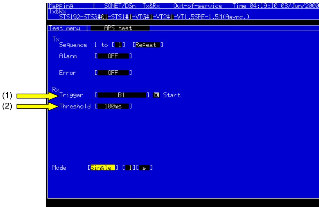
Figure 1.2 : Error/Alarm Trigger and Threshold Time Setting
