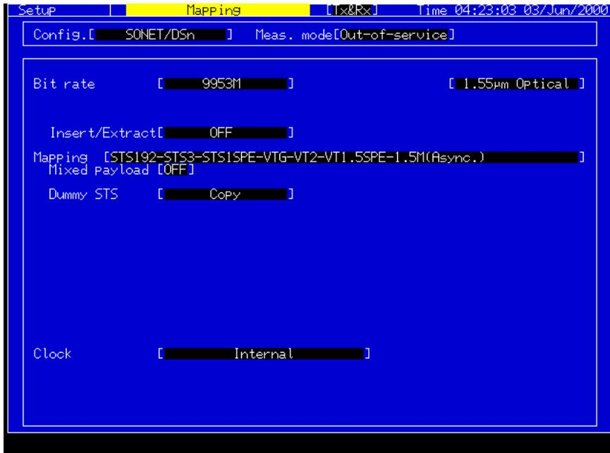
**Figure 2.3:** SETUP Main Menu Screen parameter setting
