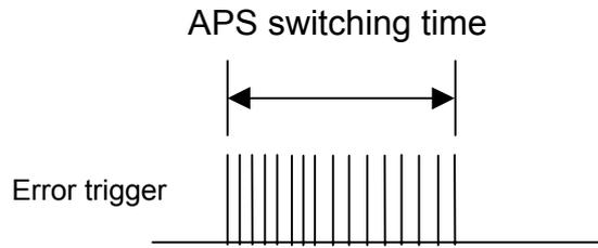
Figure 1.1 : Error Trigger for APS Switching Time Measurement
