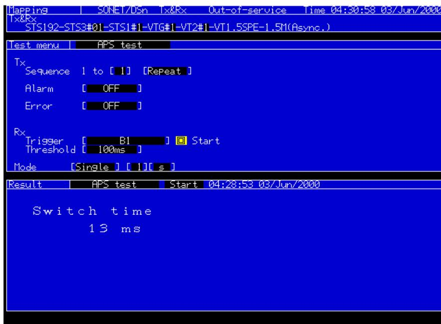
**Figure 2.7:** APS Switch Time Measurement Result
