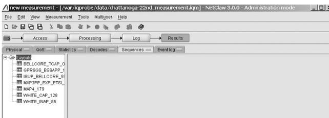
8. Using the call sequencer the network operator can find particular calls occurring in particular time periods, calls based upon calling number, called number, originating point code, destination point codes, release cause values, and call violations.
