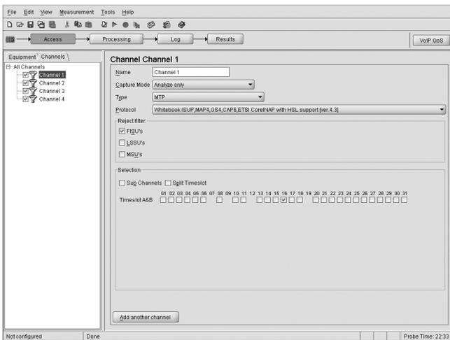
3. Start measurement by pressing the green arrow as shown below.
