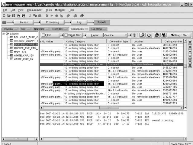
Another powerful feature of call sequencer is the filter function. The filter function can quickly allow the operator to seek a single call from a several thousand calls based on the particular field. As shown below we see a filter at work in the sequencer window searching for messages based on called number and calling number.
