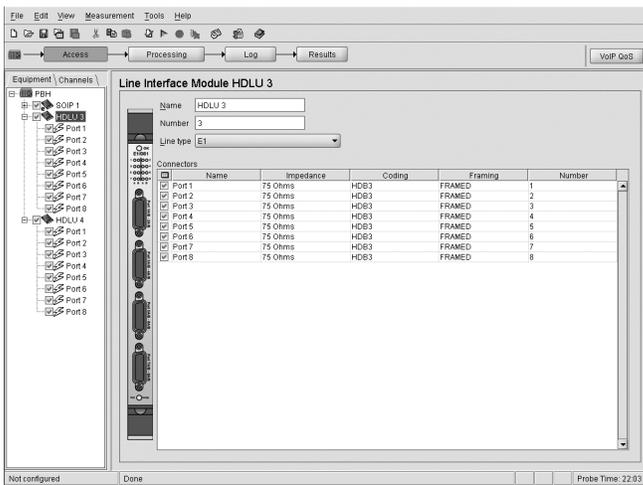
The individual channels for each T1/E1 link would be set up as given below.
