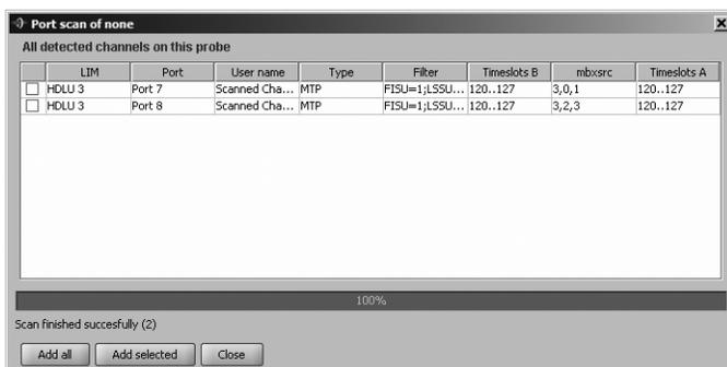
The access window is shown below which shows the 8 ports for 1 HDLU cards and what channels are configured on each port.
