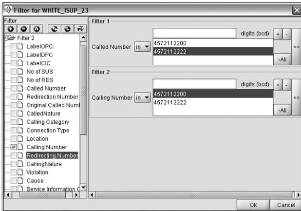
In addition to the filtering function network operators can also view a certain segment of call sequences for example the network operator is interested in all calls from phone number 410-740-7800 from 8am to 11am. This could be managed by running a time range filter in the sequence window, as given below.
