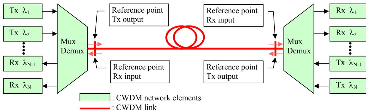
Figure 1. "Black-box" approach for bidirectional applications.
