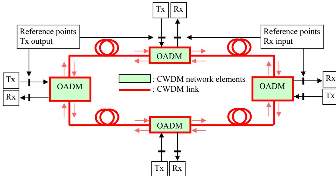
Figure 3. Ring “Black-link” approach for bidirectional applications.
