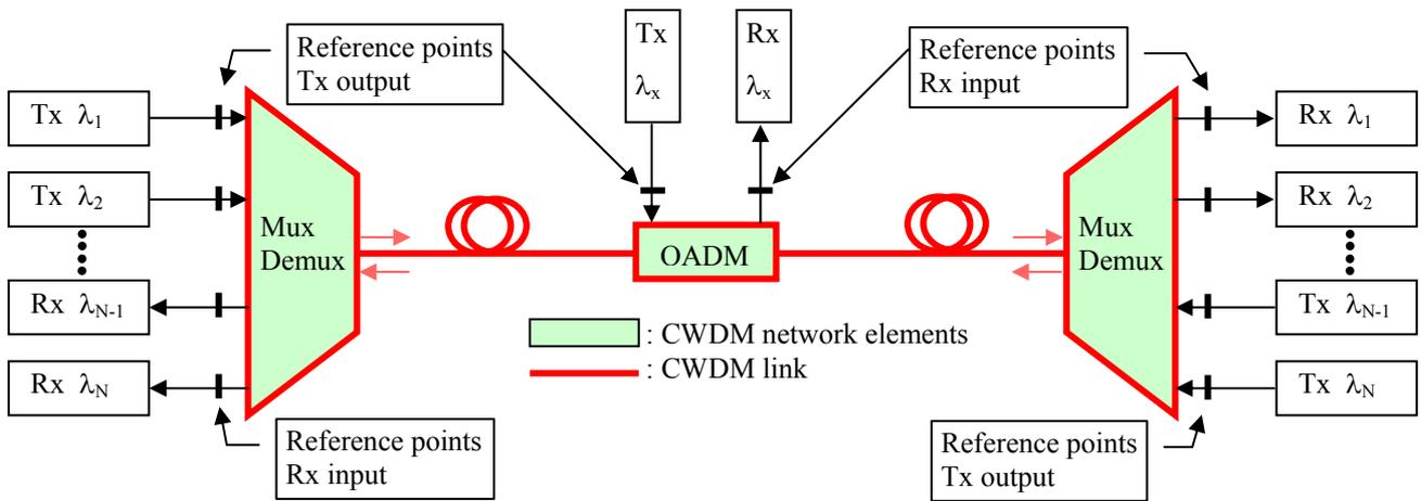
Figure 2. Linear “Black-link” approach for bidirectional applications.
