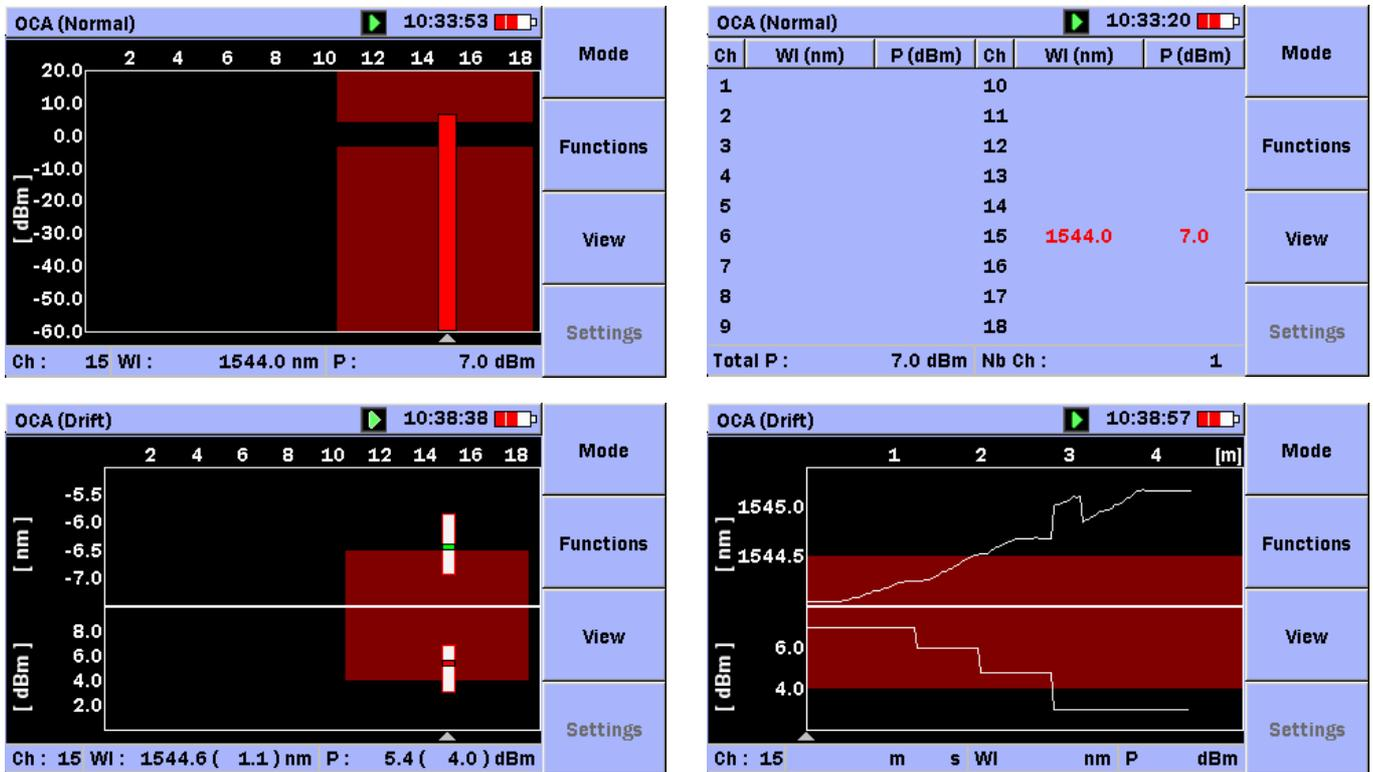
Figure 5. Alarms indicators in the different OCA displays:
