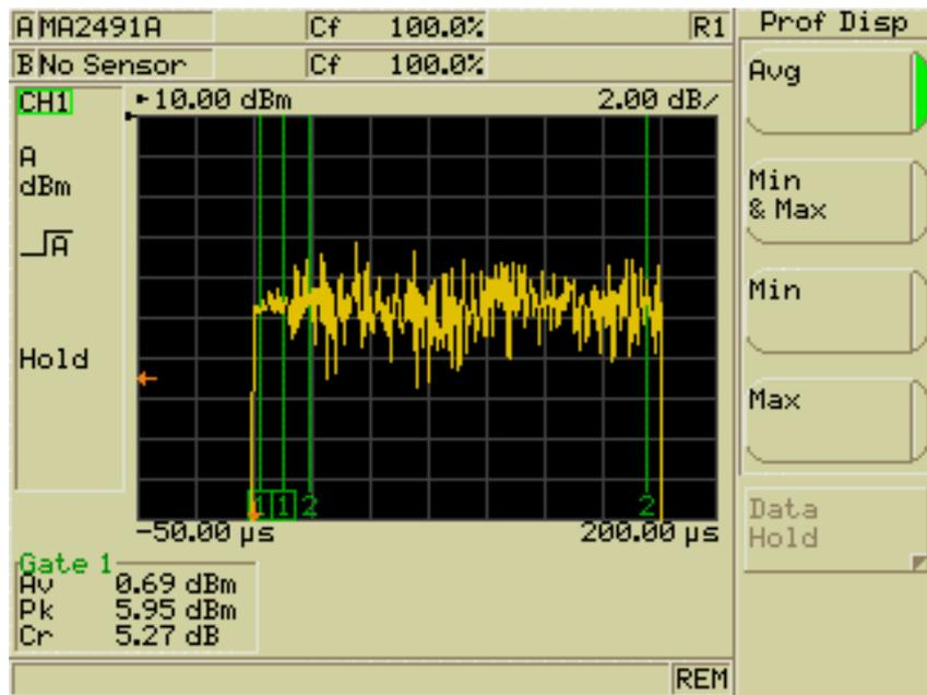
**Figure 3. 802.11a Burst with 2 gates applied**
