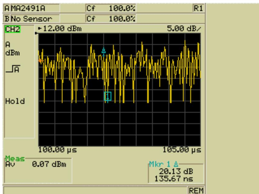
**Figure 4. A view of 5μs of the data payload in a 802.11a,OFDM, 64QAM, 54Mb/s signal**
