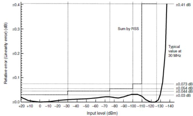
Relative error (Linearity error) at BW = 100 Hz on  $\geq 11$  MHz
