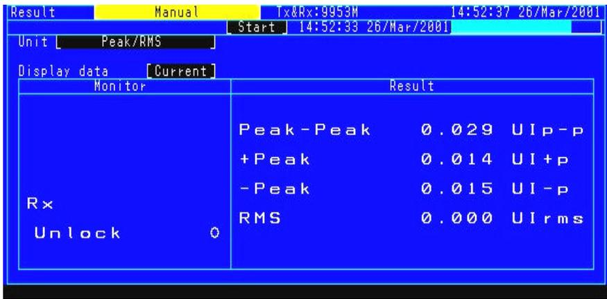
The jitter generation measurement results in the Manual mode are displayed.
