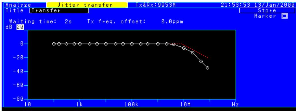
Example of Jitter Transfer Measurement Results (graph display)
