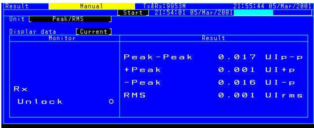
Example of Output Jitter Measurement Results (numeric display)
