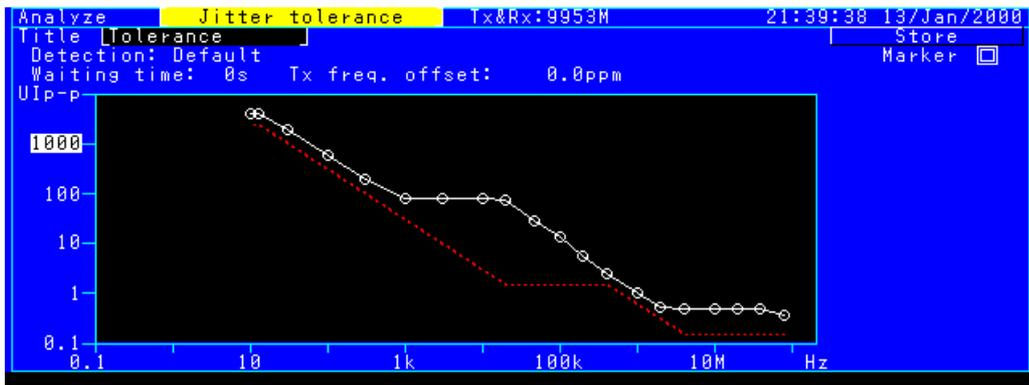
Example of Jitter Tolerance Measurement Results (graph display)
