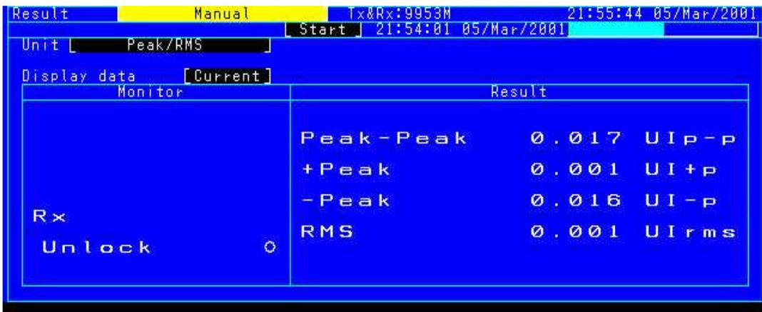
Example of Jitter Generation Measurement Results
