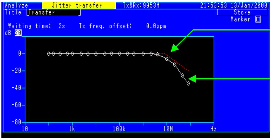
Indicates Mask for jitter transfer characteristics
